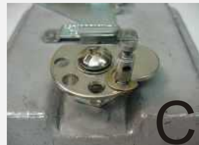
Cam & Linkpin installed.
