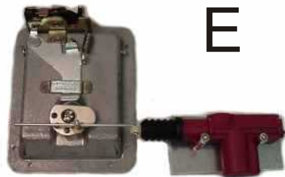
Optional Actuator mounting shown.
