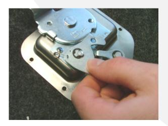
Move the spring to "Forget It" mode (hole closest to the side) and ensure the spring with the shorter end is fastened with the latch and the longer end of spring fastens to the rotating metal piece.
