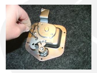
Remove E-clip with small screw driver or other appropriate tool. Note the springs location; the hole further in the middle is regular lock/unlock mode and the hole further to the side of latch is "Forget It" mode to automatically lock.
