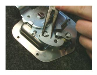
Apply E-clip to secure pieces with pliers. You can test you have forget it mode by moving metal piece and ensuring it springs back.
